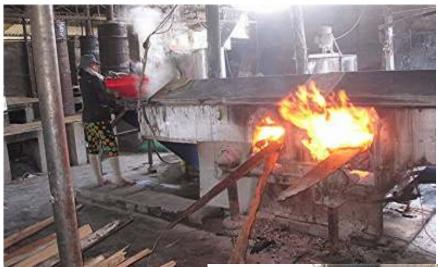
bring up images of Dante's Inferno, as shown on the left. In this picture the worker on the left is tending to the barrel of liquid rice solution that is pouring its contents on to a conveyor belt passing over the fire. The intense heat quickly cures and
